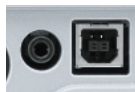
CI-V remote control jack (left) and USB connector on the rear panel ▲
