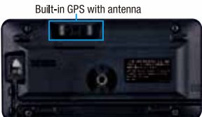
Rear side of the Controller
