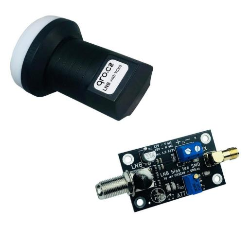
Modification of the satellite Low Noise Block (LNB) with PLL and 25 MHz X-tal.
