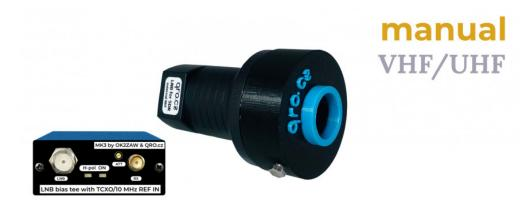
This is a new version (MK3) of the Low Noise Block (LNB) with external reference and Bias Tee box with better filtered reference frequency using X-tal filters. Crystal filters are in both the Bias Tee box and the LNB. The result is better phase noise and output (IF) signal quality even when using a worse external reference signal source of 10MHz.
