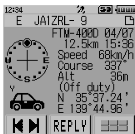
Example of display when an APRS signal is received
