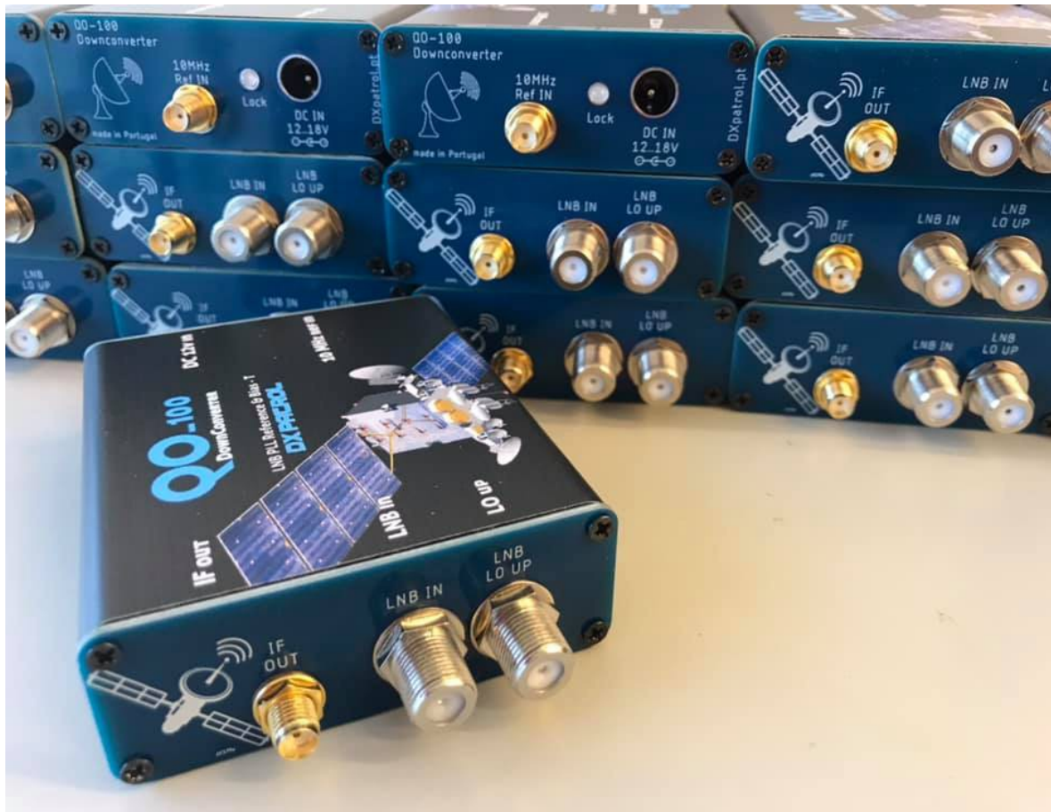
Fig 1 a complete boxed Down converter
