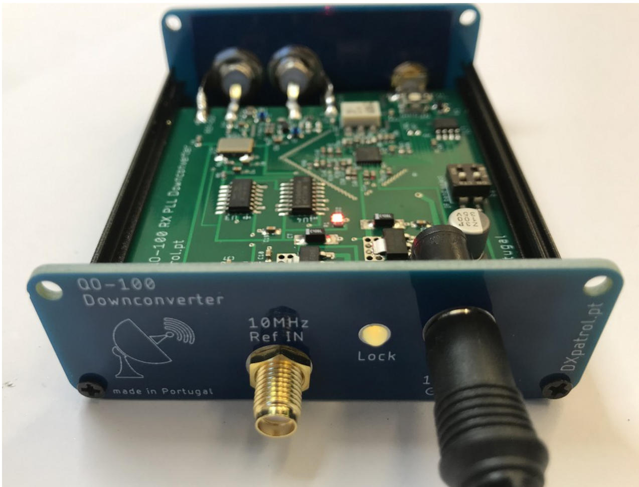
Fig 7 Orange LED = PLL LOCKED
