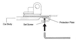
• Proper angle adjustment on trunk/hatchback installations:
