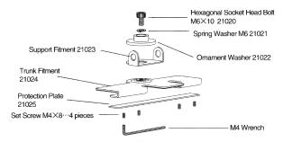
Installing Motor Drive to Bracket
