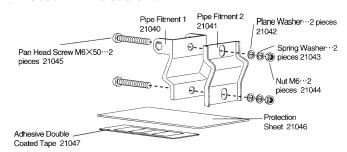
• Installing Motor Drive to Bracket
