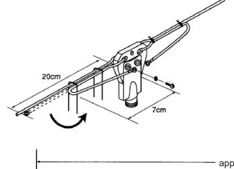
3. Connect the coaxial cable to the balun. For the purpose of waterproof, wrap the connector with self-adhesive tape, and on top wrap again with vinyl tape. Pull the self-adhesive tape to about 1.5 to 2 times its former length when wrapping.
